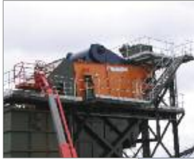
2.4m x 7m triple deck screen installed and working at Tarmac Borrás, Wrexham.
