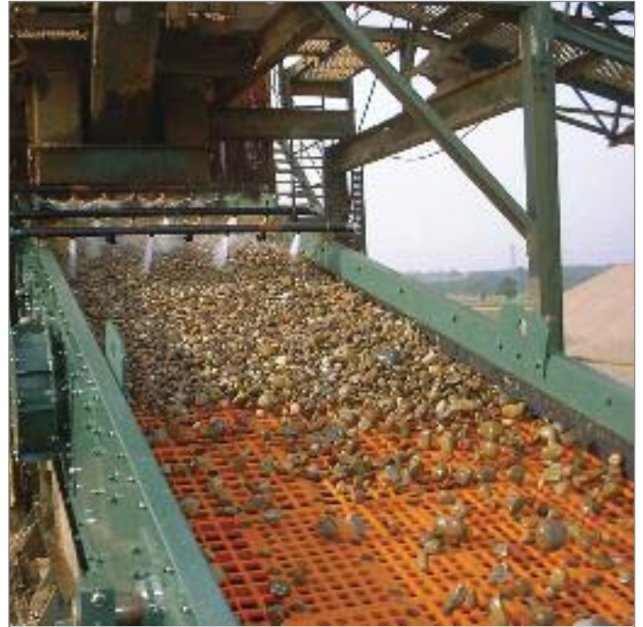
1.8m x 7m double deck feeder for Lafarge Aggregates, South Derbyshire.
