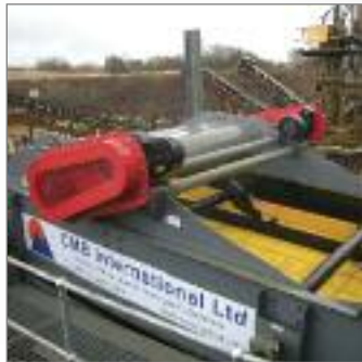
Detail of the CMB 280 vibrating mechanism.
