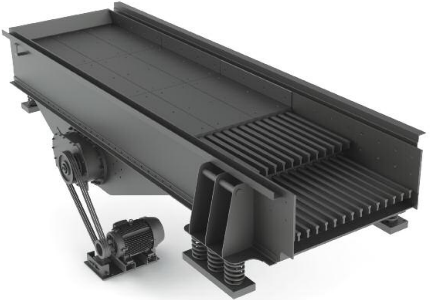
CAD Illustration of a 1.5m x 4m vibrating grizzly feeder. The feeder which has a capacity of 500 tph, has been constructed and delivered to a site in West Africa.
