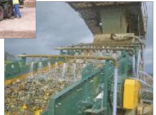
Below. 1.8m x 5m double deck screen working at Ellesmere. This screen replaced a Parker 'Rapide' unit.
