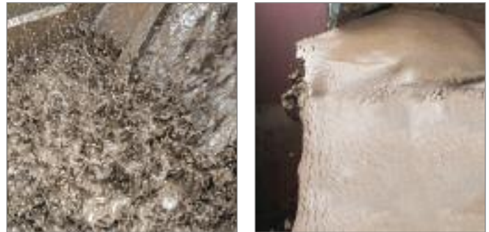
Slurry enters the dewatering screen (left) and exits as a "cake" (right), capable of being conveyed.
