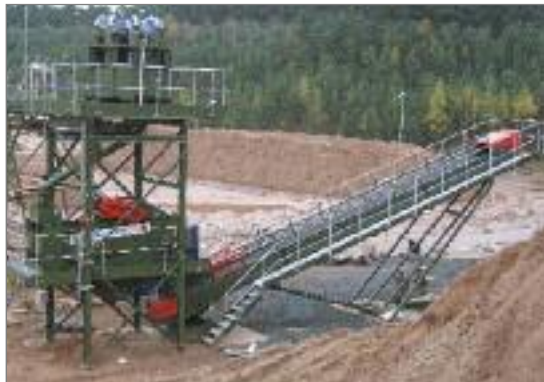
1.8m x 4.267m double deck screen working at Tarmac, Cadeby. This is the first of two screens installed by CMB.
