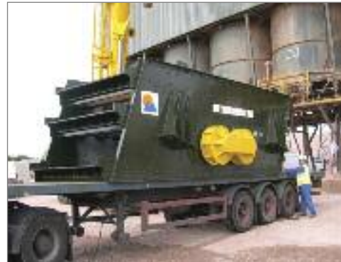
Left. 2.4m x 6m triple deck screen about to be installed in Tarmac Croxden, Stoke on Trent. This unit replaced an Alice Rippl-Flo unit.
