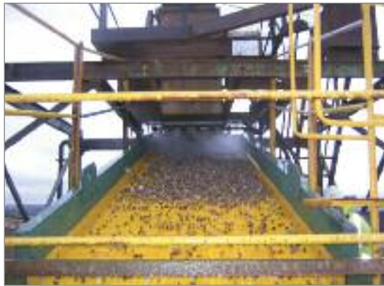
1.8m x 4.267m double deck screen working at Tarmac, Cadeby. This is the first of two screens installed by CMB.
